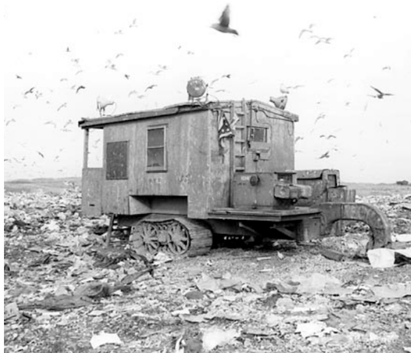
Left: The job of the bank supervisor at Fresh Kills landfill was to monitor operations at the active bank, or tipping point, of the landfill. The active bank changed from day to day, so the office would be moved on tractors to the active site. [Photographer?] / Bank Supervisor's Office, Fresh Kills / [date?] / photograph / [dimensions?]
